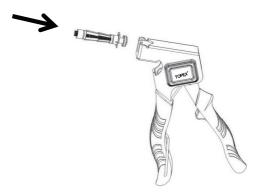
2. Screw the center gecko hollow nail of the hollow wail anchor into the head of the head u-shaped slot.
