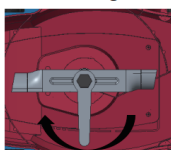
tighten the blade securing bolt
